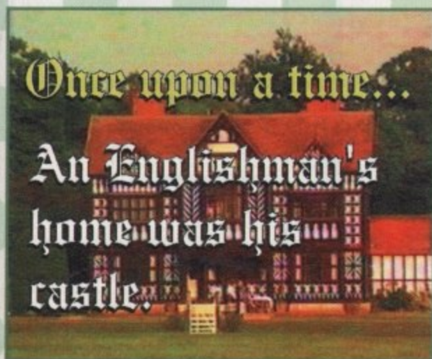
Typically, a genlock allows you to overlay graphics onto video images, as illustrated here. A text image is mixed with a video image, resulting in text on video!
